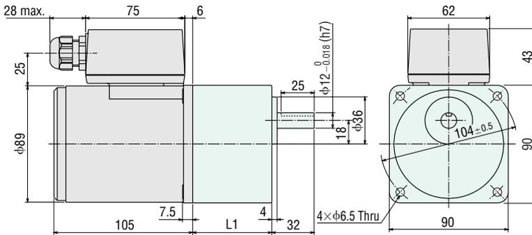
● Use cable with a diameter of  $\phi 6 \sim \phi 12$  mm.
