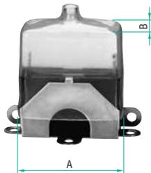
Use a capacitor cap suitable for the external dimensions (A×B) of the capacitor.
