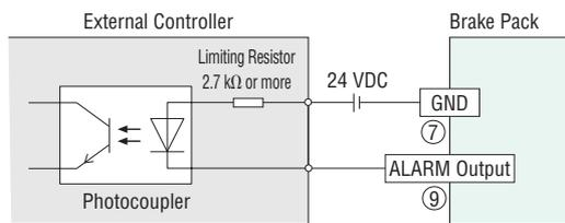
Use a power source of 26.4 VDC or less, and limit the output current to 10 mA or less.
