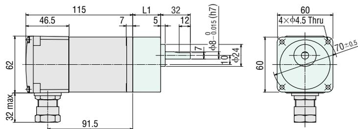
● Use cable with a diameter of φ8 ~ φ12 mm.
