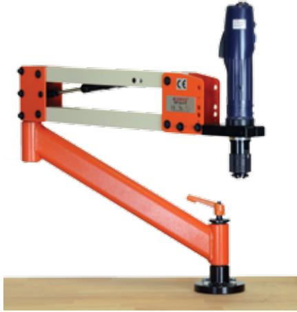
The KP-AUX1T-UTH torque reaction arm supports the weight of a screwdriver with a nitrogen gas shock and keeps it perpendicular to a work surface with its parallel arm design. Its flexibility allows it to be operated within a working range of 50–830 mm. The universal tool holder accepts a diameter of 22–46mm. Max torque is 35Nm.
