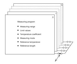
For fast object changes, RESISTOMAT® 2316 can store up to 16 measurement programs, which can be executed either by PLC, by hand or RS232 (USB, Ethernet)
