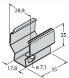
Snap bracket for mounting WLS28 work lights
