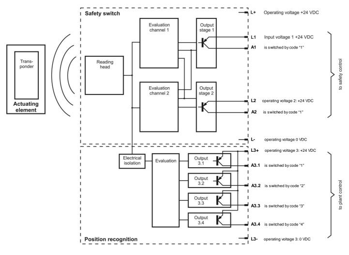
Block diagram of the basic configuration
