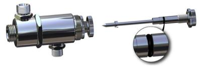
3. Unscrew adjusting needle [50] by hand and withdraw it from nozzle. Check the O-ring [51] of the adjusting needle for any damages and replace it, if necessary.
