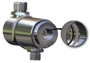
6. Check the O-Ring [15] inside the body (liquid) [10.3] for any damages and replace it, if necessary.
