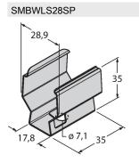
3088063 Snap bracket for mounting WLS28 work lights
