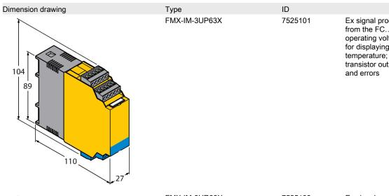
Ex signal processor for Ex flow sensors from the FC...-NAEX... family; operating voltage 20...30 VDC; LED bar for displaying flow speed and medium temperature; IO-Link device with transistor outputs for flow, temperature and errors
