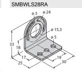
3015764 Mounting bracket, angled, metal, for WLS28 work lights, 5 mm drill holes, screw set included
