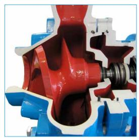
Sectional view of Impeller Housing Assembly
