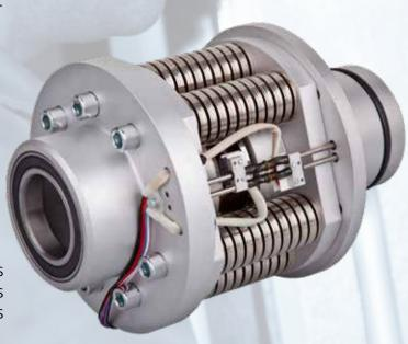
Should a malfunction occur and the previously selected load be exceeded, the electric actuator will switch off and that before damage to the entire system will occur.
