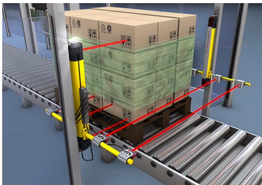
Figure 5.4: Access guarding on the roller conveyor with timing controlled 4-sensor muting (MLD 535 with pre-mounted muting sensor sets)
