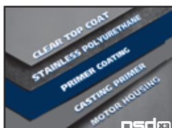
NSDX3 on Cast Iron
