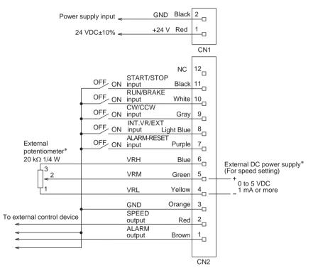
\* Connect either the external potentiometer (accessory) or DC power supply for the external speed setting.
