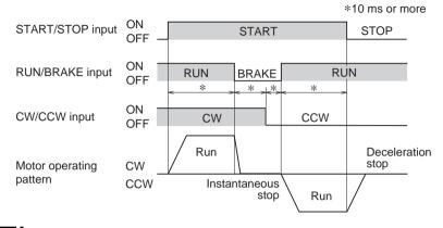
Note Once the motor stops, the output shaft will become free.
