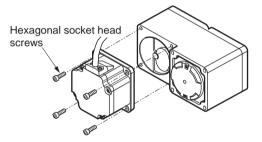
2. Using the pilot sections of the motor and gearhead as guides, install the motor to the gearhead and tighten the hexagonal socket head screws. At this time, the motor cable position can be changed to one of three 90° directions.
