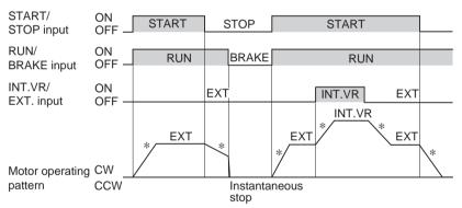
\* The motor starts and stops over the time set by the acceleration/deceleration time potentiometer.
