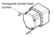
2. Using the pilot sections of the motor and gearhead as guides, install the motor to the gearhead and tighten the hexagonal socket head screws. At this time, the motor cable position can be changed to a desired 90° direction. When installing the gearhead, slowly rotate it clockwise/counterclockwise to prevent the pinion of the motor output shaft from contacting the side panel or gear of the gearhead.
