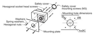
• Using the rear side as the mounting surface
