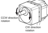
• Combination type hollow shaft flat gearhead
