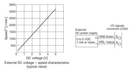
\* Indicates the speed of the motor alone. The speed of the gear output shaft of a geared type or combination type is obtained by dividing the motor speed by the gear ratio.
