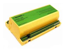
The ETN-40 is a distributed ETN slave module, with 16 optoisolated digital inputs, active at 24 V<sub>DC</sub> or GND, and with 16 relays outputs. It is completely managed by an ETN master controller. The ETN-40 receives the state of the 16 digital outputs from the master controller and sends it back the 16 digital inputs state.
