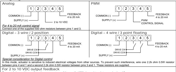
For any of above wiring configurations, connect one of the supplied 500 ohm resistors between pins 1 and 5.
